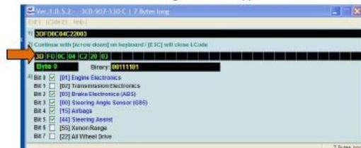
In line 3, click each code (3D, FD, 0C, etc) in turn until a screen appears in which Bit 7 shows 69-TRAILER
