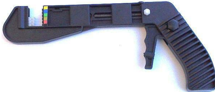
Putting a 3-way splice socket onto a pair of host wires
