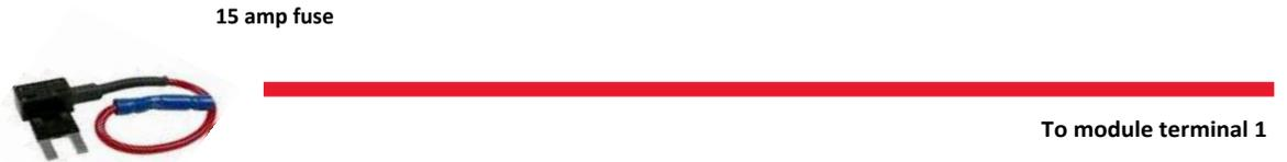
To supply both the 12N and 12S, use the orange cable, one PowerTap and 15 amp fuse, and the heavier, black cable the other PowerTap and the 20 amp fuse. Connect the PowerTap to one end of each cable and connect the other ends directly to Terminals 1 (orange) and Terminal 2 (black) of the CANbus module. Select suitable fuse positions in the fusebox to insert the PowerTaps.
