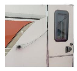
The device is fitted between the release lever and a hook inside the door
