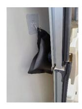
With the door in the retained position the lift bag is inflated enough to be firm between the door and the caravan side. This is the "ready" condition.
