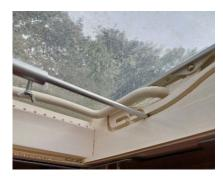
When the rooflight is closed, the Windjammer stores neatly within the rooflight frame
