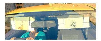
The visor extension fits to the front of the pulled-down visor.
